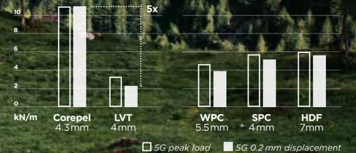
A proven advantage (ISO 24334:2019) - Corepel's exceptional strength has been confirmed using tensile strength tests. When two locked panels are pulled apart, Corepel panels withstand a force that is up to 5x higher than panels with LVT, WPC, SPC and HDF core.
